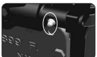
Draft Sensing Spindle
